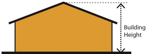
Figure 2. Measurement of Building Height
